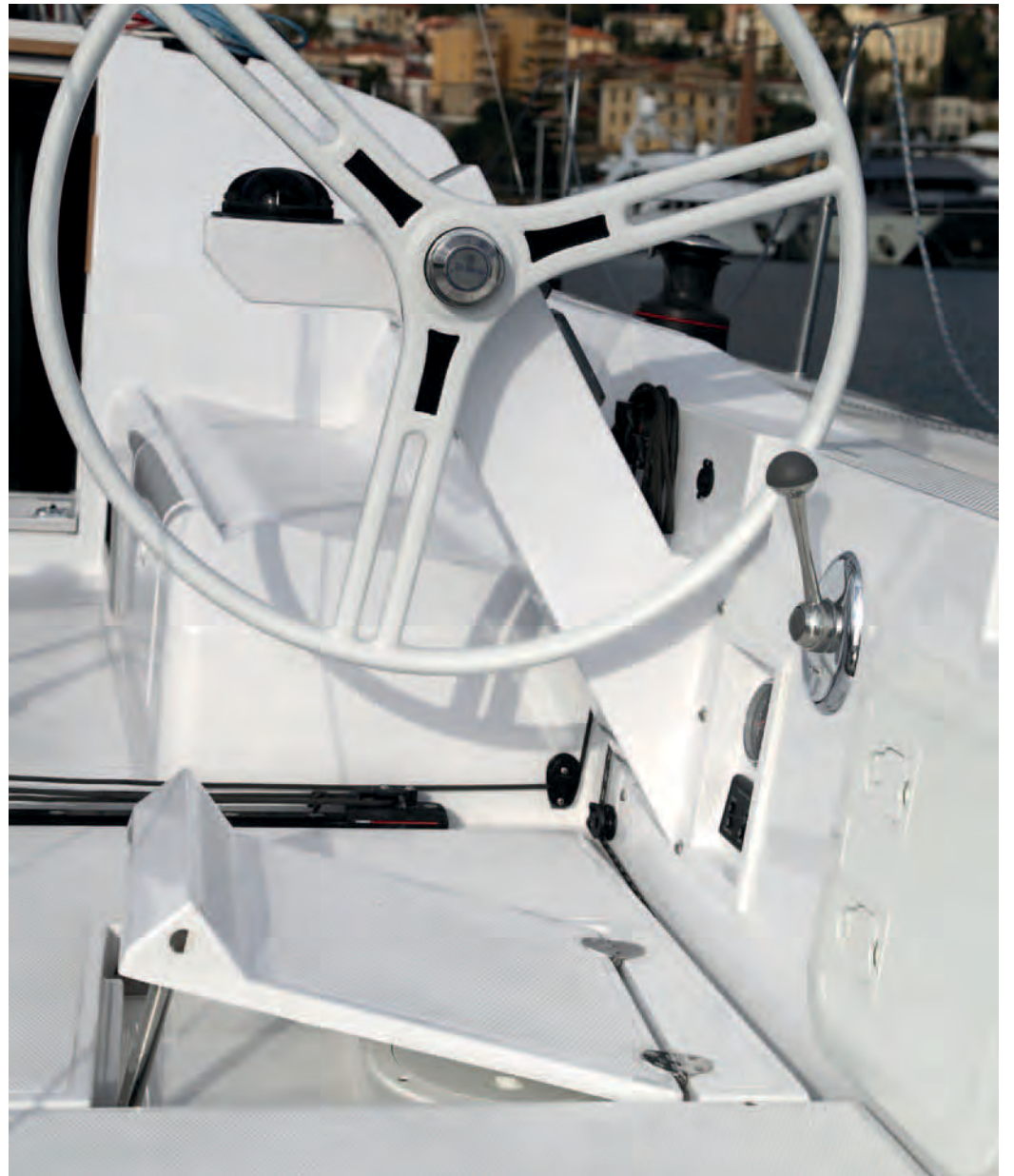
Helmsman's foot support for safe and comfortable steering when heeled.
