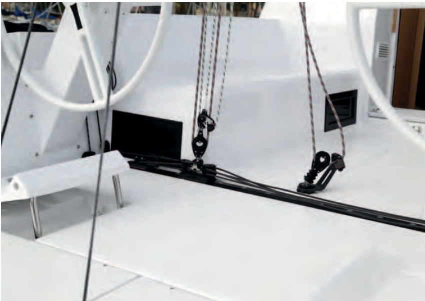
Recessed mainsheet traveller and two additional portlights in aft cabin for more light and air.
