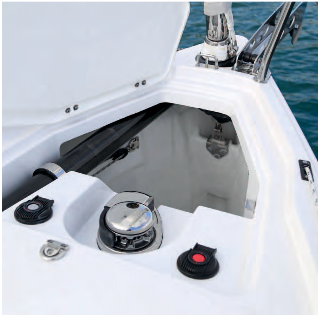
Anchor locker with removable anchor roller, through-deck furler and access to the gennaker pole.
