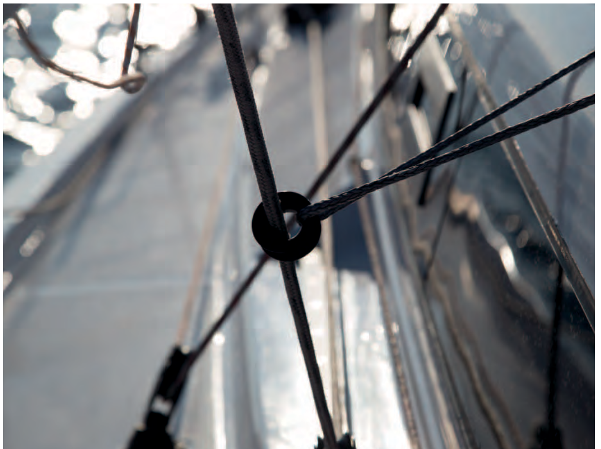
Barber jib in haul for achieving better angles upwind.
