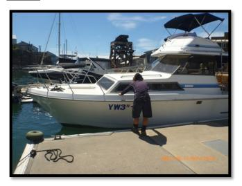
The GRP deck areas are well constructed and include non-skid surfaces. The foredeck area is accessed via walkways either side of the main saloon. The handrails are solid and well positioned.
