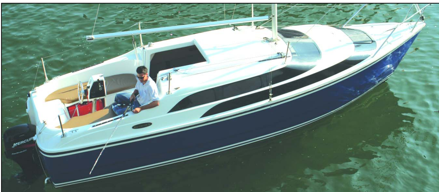
Here is another view of the boat, showing the deck and cockpit layout, as well as our fisherman trying his luck. The hatches can be secured to keep water out of the inside of the boat. The cockpit is self bailing. The cockpit floor is above the water level, so any water that comes into the cockpit simply drains out through the open transom. This is both a convenience and a big safety factor. (A swamped boat is no joy, and having to bail out a cockpit full of rain water is no fun either.)
