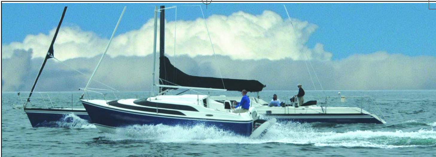
The MacGregor 70 may sail faster, but the 26 can nearly double its speed under power. Here you see the two boats going full throttle. The 70 is doing about 13 mph (very fast for a sailboat), and the 26 is doing over 20. The 26 is burning a lot less fuel.
