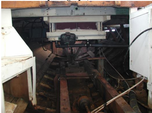
The motor space and remnants of the vee drive below and rot in the top port planking at the mizzen chain plates.
