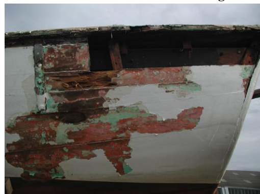
The motor space and remnants of the vee drive below and rot in the top port planking at the mizzen chain plates.
