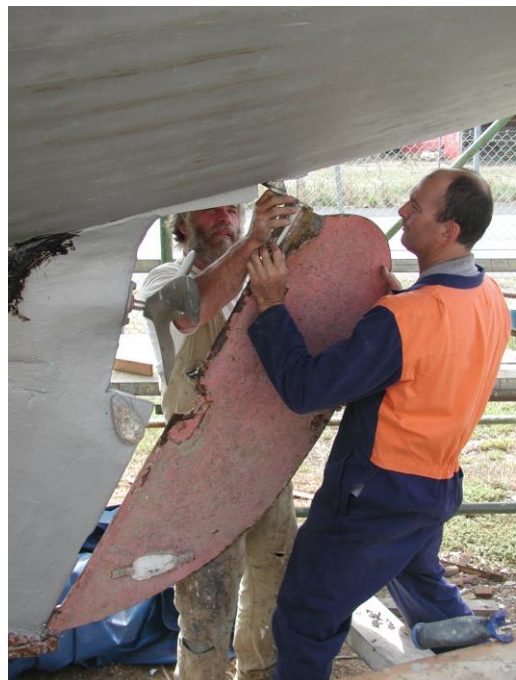
Brett and Laker Engineering's Fitter reassembling the rudder
