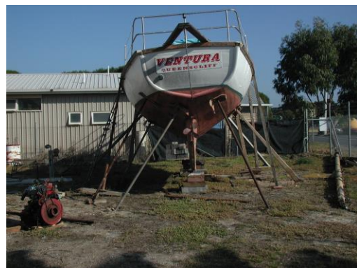
Craning out and in the Yard. The lean was a result of incompetent propping. In the right-hand photograph, the Buch motor can be seen on the left and the main mast on the right.
