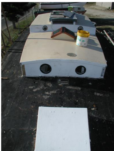
The deck and deck planking ready for fixing ply and epoxy fibreglass and priming of the Bilge.
