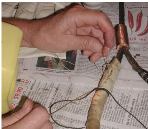
Sandra Crockett working late at night on leathers on the shroud loops, one of the many jobs for which the time was underestimated, started too late but nevertheless finished just in time for re-stepping the masts.
