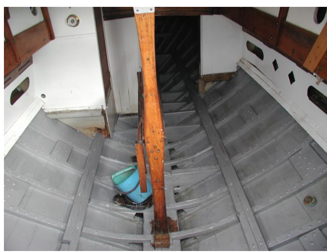
The deck and deck planking ready for fixing ply and epoxy fibreglass and priming of the Bilge.
