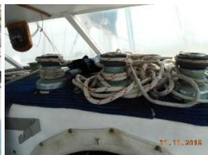
Five self-tailing *Maxwell* halyard winches, one of which is 12v powered, are mounted on the coach house forward in the cockpit and five self-tailing sheet winches *Arco 52* and *Barlow* are fitted on the aft bulwark capping in the cockpit. A lightweight spinnaker is carried and can be rigged off either bow in light airs. Two headsails with UV weather strips and a mainsail in a zippered boom bag are rigged to the vessel.
