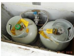
Two 8.5kg LP gas bottles are stowed forward in the cockpit in a self-draining locker and plumbed to supply the galley stove. A closing valve is fitted in the line under the stove. Outboard fuel is stowed in several PVC canisters in the starboard foredeck locker.
