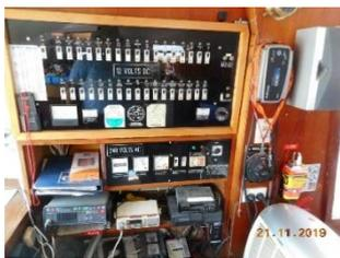
The vessel is wired for 240vAC and 12vDC. The AC system is powered by a connection to shore mains through an IP34 fitting forward in the cockpit to a distribution panel in the saloon. The supply is properly metered and protected with an earth leakage circuit breaker. A 1.5kW 12/240v inverter located under the distribution board also provides limited AC power when the vessel is at sea and an isolator switch is fitted for selecting shore or ship supply.
