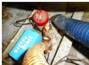
Automatic 12v submersible bilge pumps are fitted along with manual pumps that draw from the machinery space and amidships compartments. A portable backup manual pump is also carried which can draw from any hull compartment.
