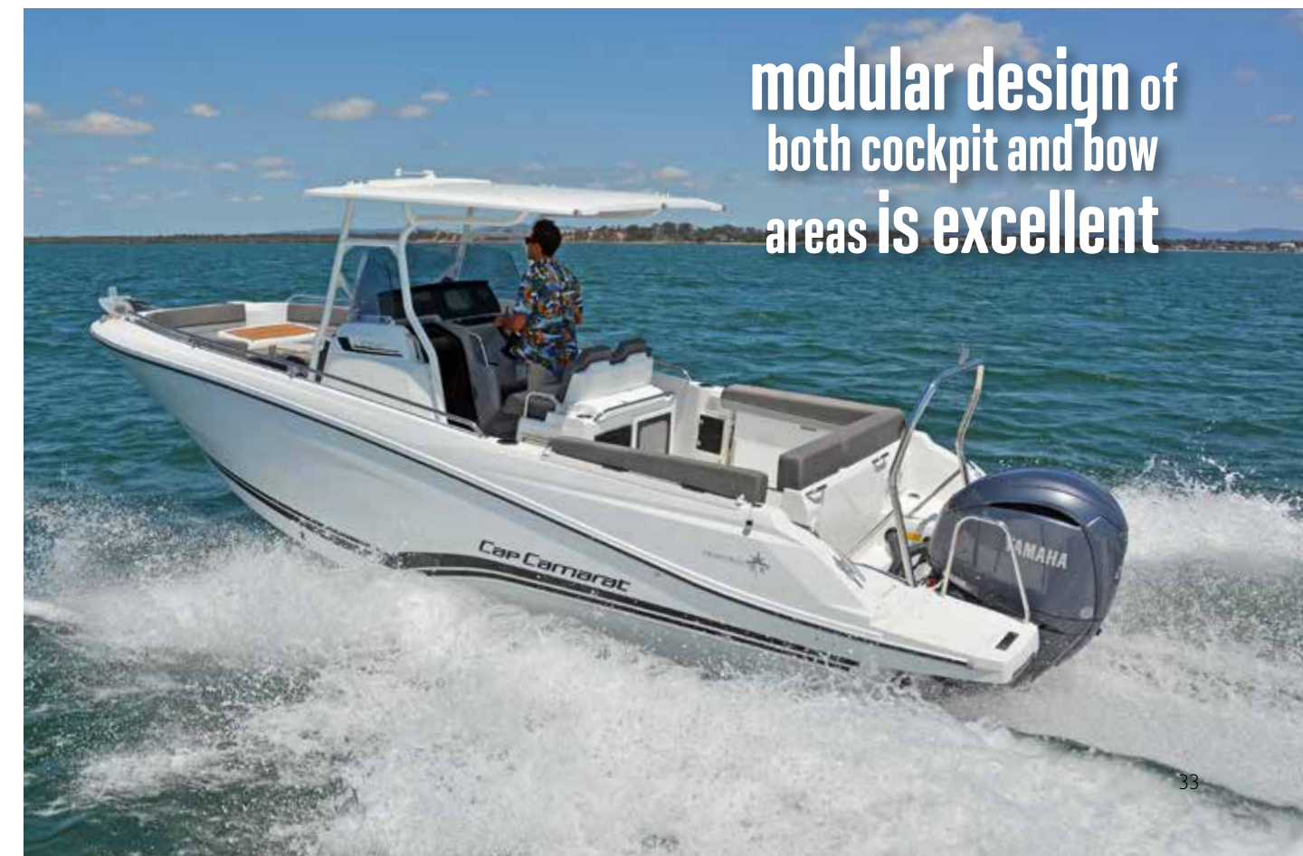
Below: The hull is designed for a single ultra-longshaft outboard to a maximum of 300hp.
