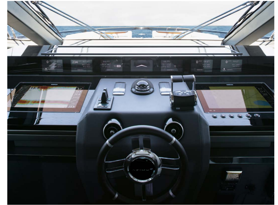
The bridge was produced in partnership with Simrad-Naviop and has a single ultra-wide screen displaying key monitoring and navigation information, a mix of video sources and clusters of content. Accessing this information is easy with a choice of commanders or two touch screens duplicated by a pair of physical joggers for extra redundancy and safety.
