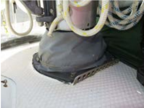
Mast boot without deterioration
