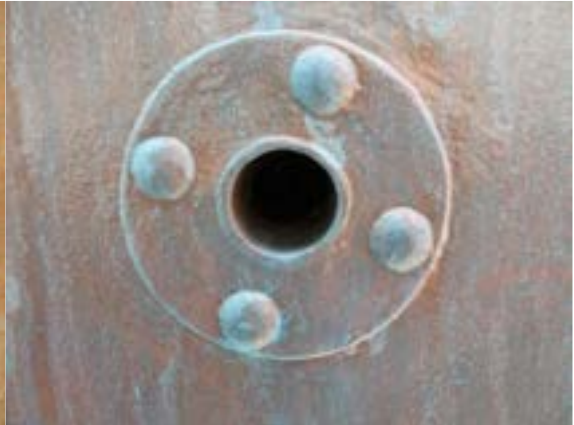
Through hull necks without wastage
