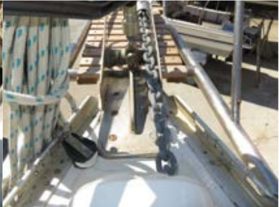
Anchor roller without damages
