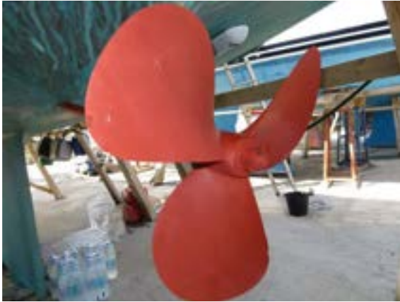
Propeller without damages to the blades
