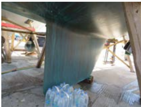
Keel externally intact
