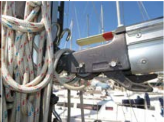
Mizzen boom gooseneck without fracture
