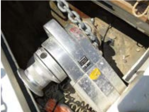
Anchor windlass casing without wastage
