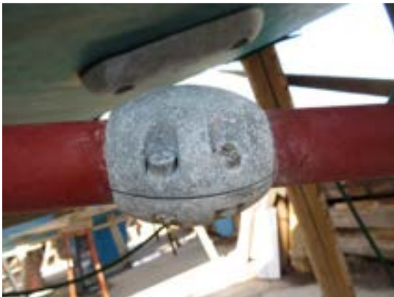
Shaft anode new
