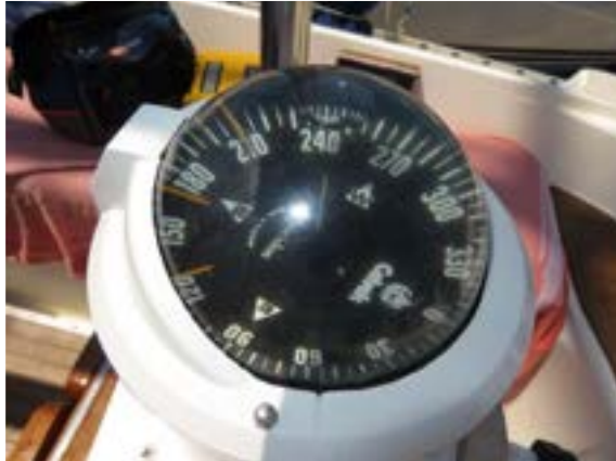
Magnetic compass with small bubble
