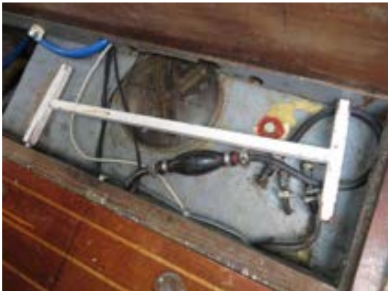
Fuel tank externally intact
