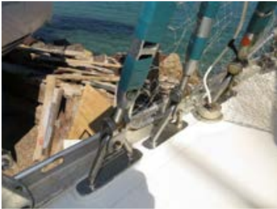
No crazing or delamination in way of shroud chainplates
