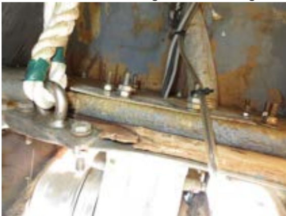
Anchor windlass securing bolts not corroded
