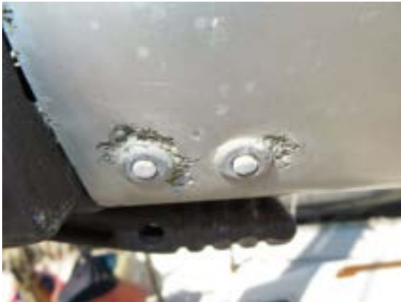
Minor galvanic corrosion at bimetallic interface of aluminium and stainless
