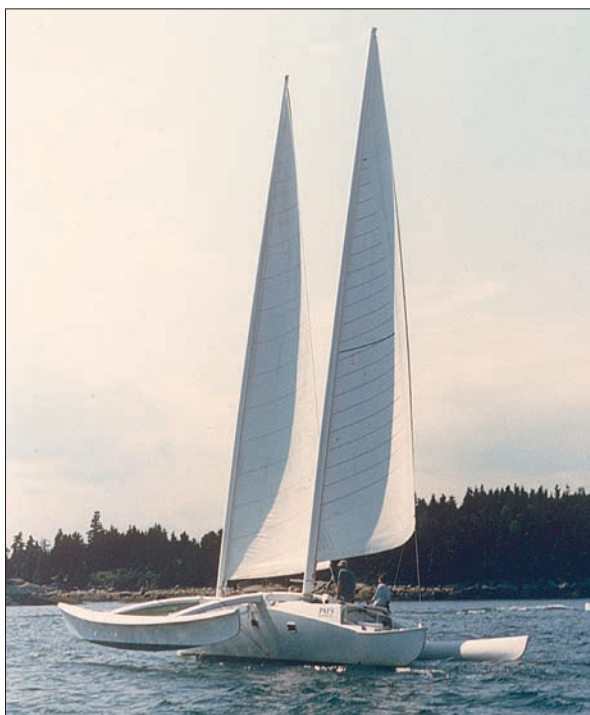
Dick and Pat Newick's own cruising boat, the 51' (15.5m) Pat's, was launched in the late 1980s and is now in Europe under new ownership. Auxiliary power is an 18-hp (13.4-kW) Volvo. Accommodations are spacious enough to permit a pair of double berths.
