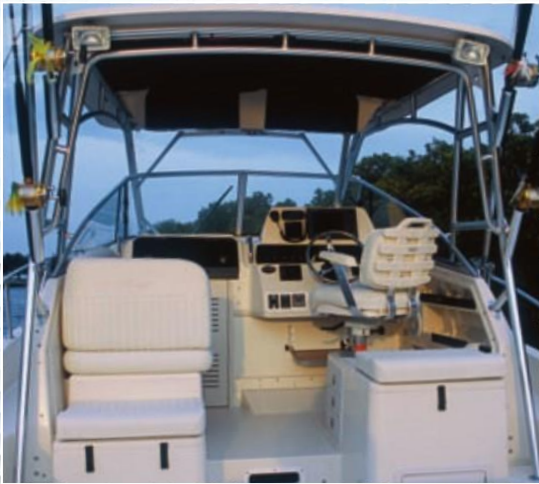
§ Cabin model hardtop with lockable radio box(es), spreader light(s), side rod holders and overhead storage net (optional models 22'-25', standard 29'-36')
