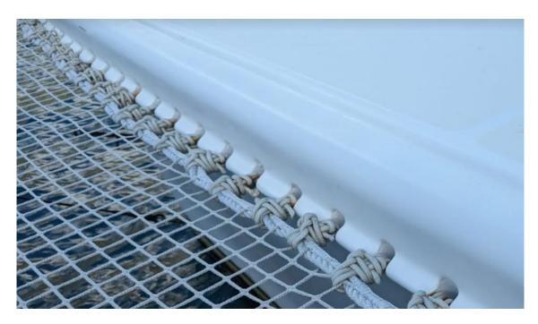
The solent rail was removed, all holes clogged. The rail was re-installed on a new epoxy structure.
