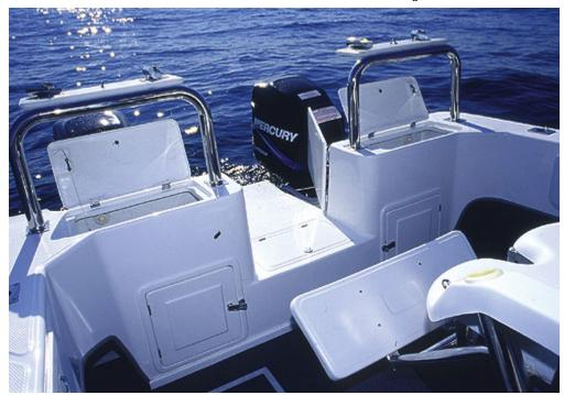
Have a look at the photographs of the false transom area — with its livebait wells and marlin gate, as well as storage lockers — and you will agree that this craft has everything a ski-boat angler could desire. By the way, the rounded aft corners provide sufficient area to situate a Luna tube in each corner, if required.
