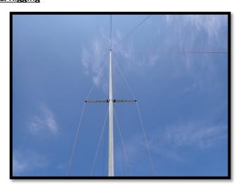
Rig configuration Sloop – keel stepped - 1 spreader masthead
