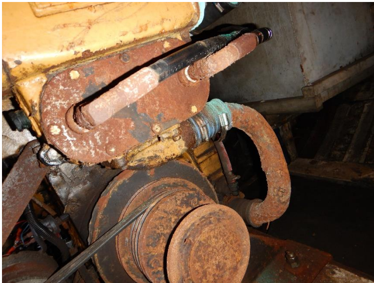
Deterioration of hoses and clamps
