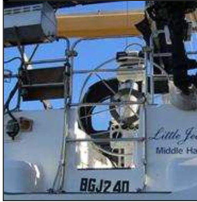
2.14 Item 1(Picture) Access ladder as Gate aft Access ladder acts as a Gate when not being used.
