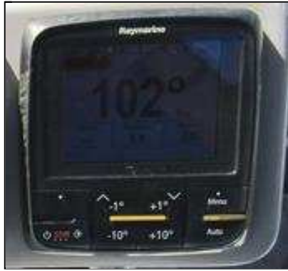
9.9 Item 1(Picture) Auto Pilot Auto Pilot control head i7
