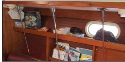
10.13 Item 1(Picture) Stbd chain plate rods
