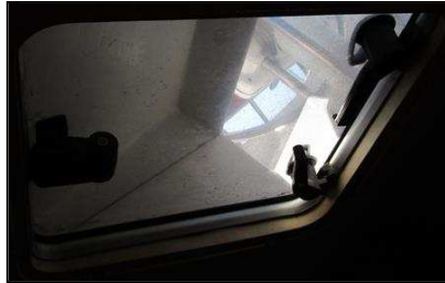
2.6 Item 3(Picture) W/T Escape hatch from after cabin to cockpit
