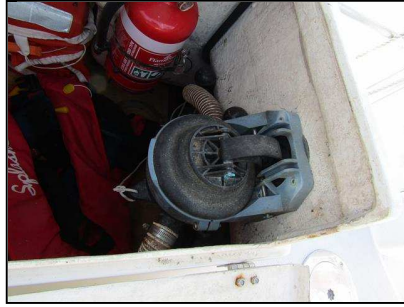
6.4 Item 1(Picture) Manual Bilge pump Two manual bilge pumps aft - steering flat.
