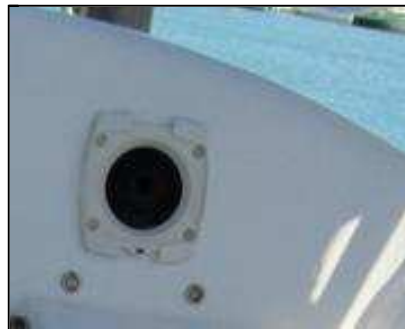
6.3 Item 1(Picture) Manual Bilge Pump in the stbd side lazarette
