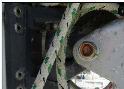
10.1 Item 1(Picture) Gooseneck connection & pin Boom gooseneck connection & pin in good condition
