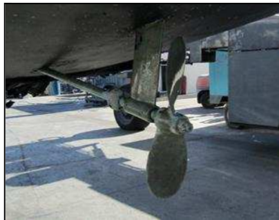
1.9 Item 1(Picture) Propellor shaft & cutlass bearing Propellor Shaft c/w Cutlass bearing and propellor
