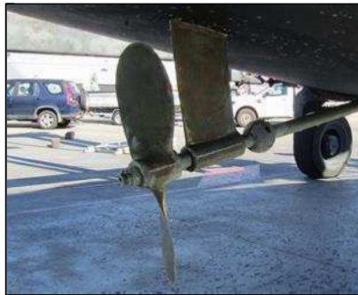
1.8 Item 1(Picture) Propellor Propellor coated with PROPSPEED
