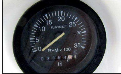
6.2 Item 3(Picture) Hobbs Meter 3193.5
