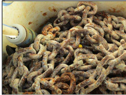
5.16 Item 1(Picture) Anchor Chain in Locker
