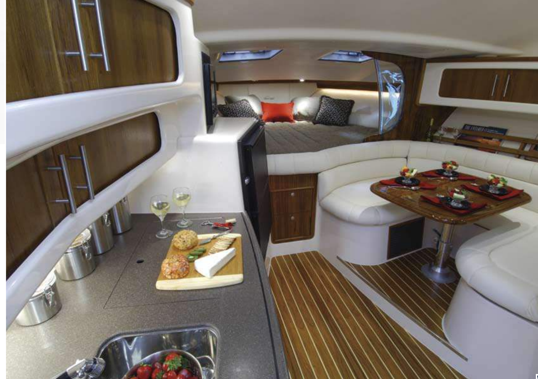
5 - Main cabin includes teak and holly sole, seating for four at teak dinette table, variable accent lighting, 16,000 BTU air conditioning with zone cooling, expansive forward berth with storage and privacy curtain, and teak tambour enclosed storage areas.
