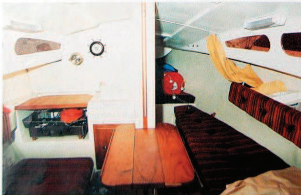
The dinette has two dropsides and fits between the bunks to seat four or more in comfort
