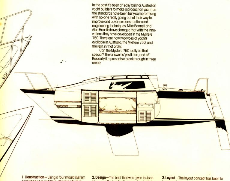
1. Construction — using a four mould system consisting of ① Hull then attaching to that ② Hull liner, ② Cabin liner, and ④ Cabin and deck mould. This method of interlocking shells produces a very rigid framework, and a strong, stiff yacht. Now, such a system also reduces the total weight of the yacht hull, so the Mystere is also ahead on lightness, and hence responsiveness.
