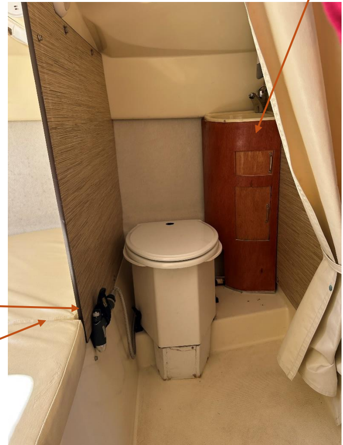
Head / Toilet (0.7m wide cubicle) (composting + fluid direct discharge)
