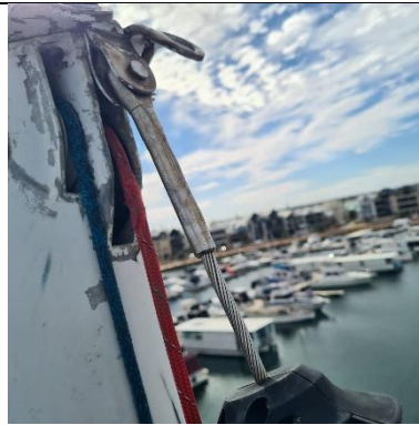
Forestay damage from halyard wrap
