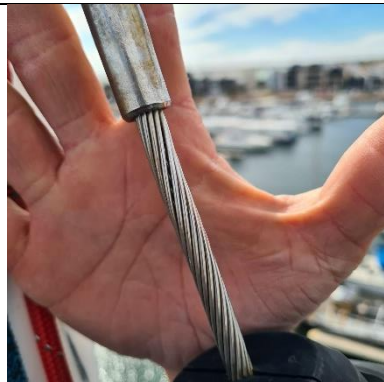
Forestay damage from halyard wrap
