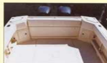
Aft cockpit with fold-down motorwell bulkhead
