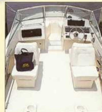
Cockpit forward with standard port and optional starboard sleeper seats
