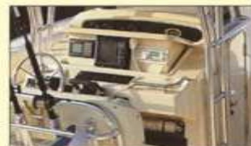
Console with electro-mechanically operated electronics enclosure
