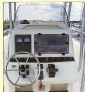
Console with lockable electronics box
