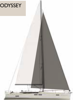
Large overlapping genoa / Génôis à fort recouvrement / Genua in starker Überlappung / Génova con mucho recubrimiento / Genoa a forte recupero
